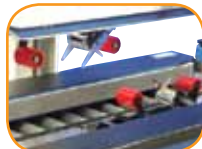
Offset tape heads process 2" high cases
